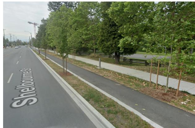
In Saanich, Shelbourne Street between North Dairy Road and Pear Street are protected bicycle lanes constructed at the same grade as the sidewalk and separated from motor vehicles by a normal concrete curb and boulevard.
