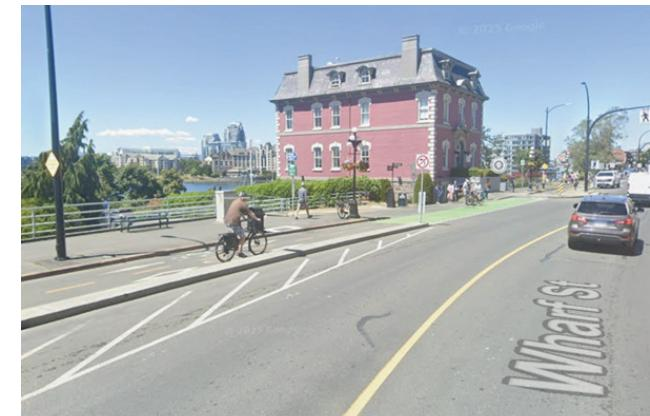
In Victoria, Wharf Street is an example of a bi-directional protected bicycle lane using cast in place concrete curb and delineators.
